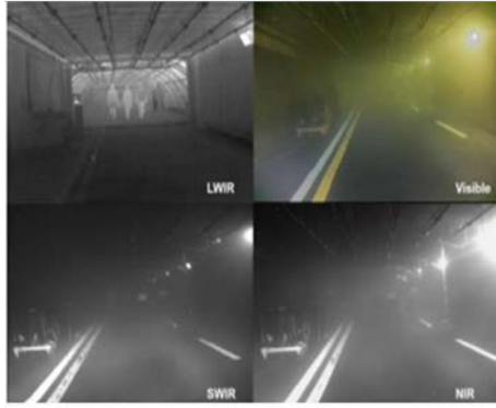
[Example of images recorded in the fog tunnel with the four different Cameras]
